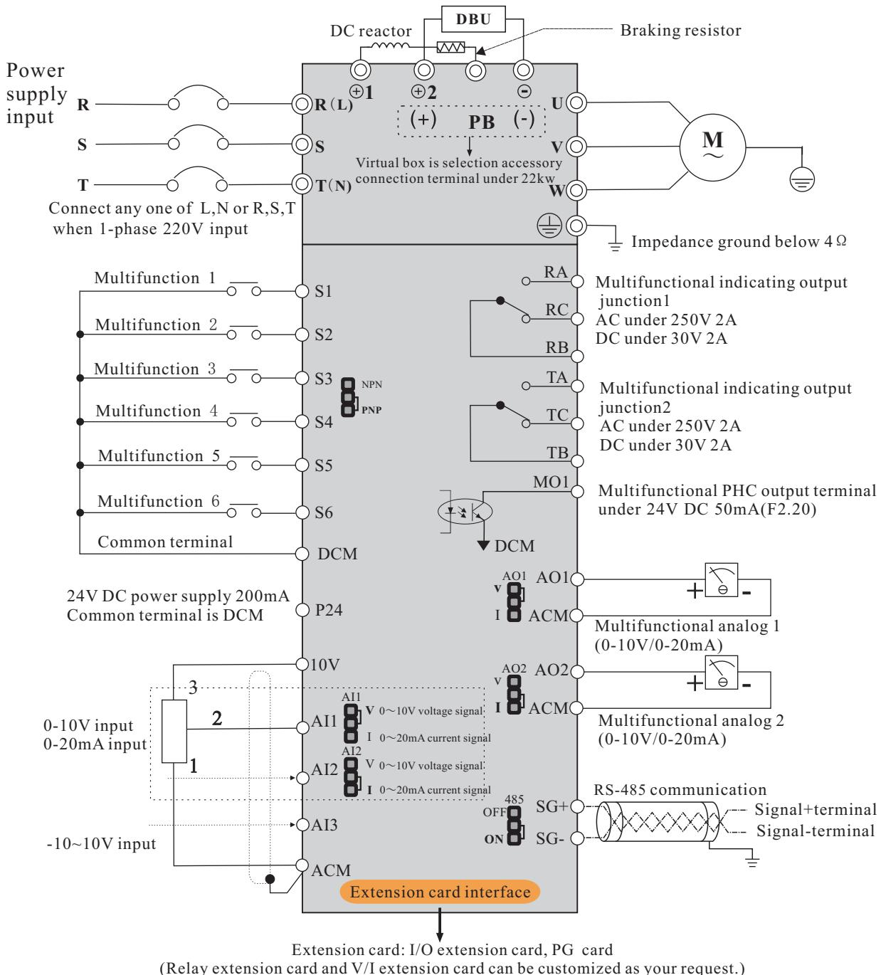
**Notes:** The general type inverters of 22KW and below have built-in brake unit, brake resistance (+) and PB terminal; (+) and (-) terminals are the plus or minus terminals of inverter's DC bus. Reserved direct current reactor connection terminals above 22KW,  $\oplus 1 \oplus 2$ ,  $\oplus 2$  and  $\ominus$  terminals are used to connect energy feedback unit or brake unit.
